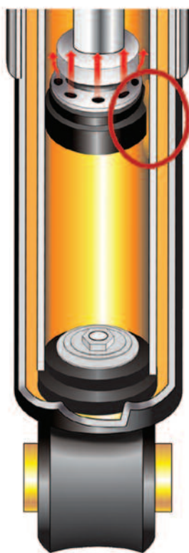
Damage to the piston seal causes the oil to flow past the piston in an uncontrolled way which decreases oil pressure. The lowering of the pressure reduces the cushioning force.
