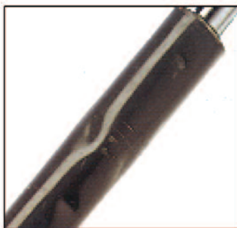
Damage to the body can be caused by an accident or road debris. Damage prevents or slows down the piston rod as it goes back and forth.
