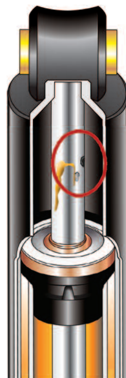
Damage to the piston rod can be caused by corrosion or tools which causes the seals to be damaged and oil leakage to occur.
