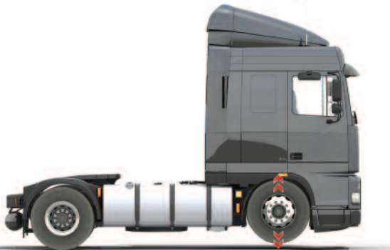
Excessive tyre bounce on bad road surfaces.
