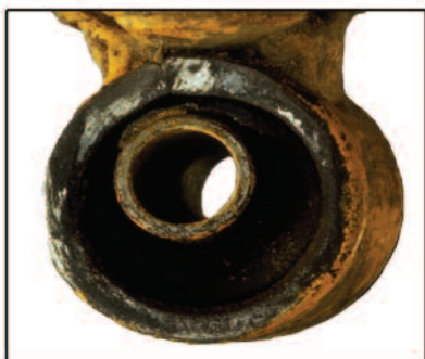
Damaged mounting can be caused by overloading a vehicle.
