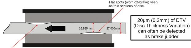
Thin sections of rotor slip between pads with less resistance than thick sections
