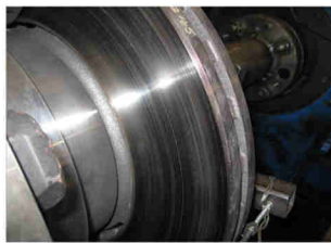
Outboard Disc after 200 stops
