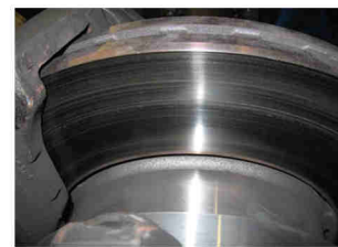
Outboard Disc after 400 stops
