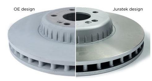
achieve the same tensile strength, the cast iron hub needs to be a minimum of 6mm.
