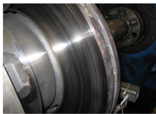
Outboard Disc after 200 stops
