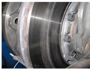
Inboard Disc after 400 stops
