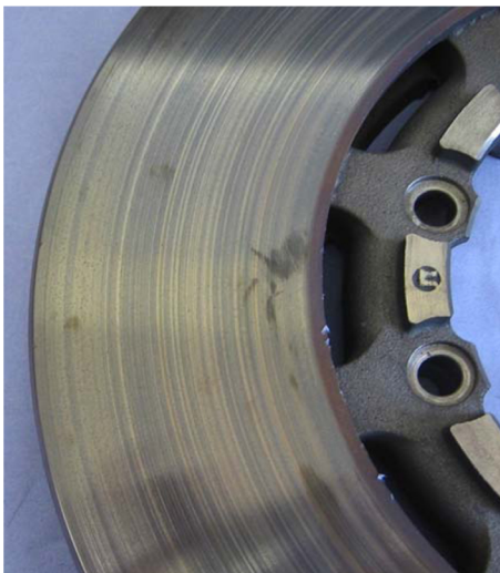
Inboard Disc after 500 stops - Test completed
