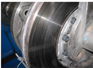
Inboard Disc after 200 stops
