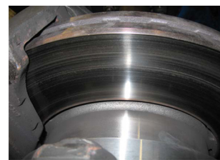
Outboard Disc after 400 stops
