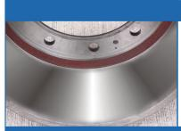
Polished drums can be identified by a mirror-like finish on the braking Surface. This problem can be remedied by lightly sanding both the lining and brake drum surface with some medium grit emery cloth. The brake system should be checked for lightly dragging brakes and the linings should be checked to ensure the correct material is being used.
