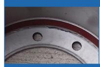
This problem occurs when there is interference between the hub and drum mounting surface, due to incorrect seating of the drum on the hub during installation, a damaged hub, or a build up of corrosion on the hub. Prior to brake drum replacement the hub should be visually checked and any defects rectified, by either cleaning up the hub or replacing where necessary. If any cracks are identified in the bolt circle or mounting surface the drum must be replaced.
