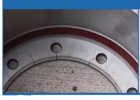
This condition is caused by interference between the hub and drum mounting surface during installation as a result of using the wrong drum for the application or improperly cleaning the hub piloting surface prior to drum installation.
