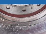
This problem is indicated by defined grooves in the braking surface of the drum and excessive brake lining wear. These grooves are caused by either the brake linings being completely worn out causing a metal to metal situation, or a foreign body finding its way inside the brake drum
