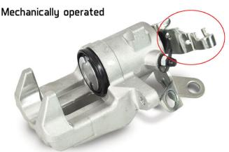
This type of caliper is used for normal pedal braking and the piston is operated hydraulically. However it is also used to operate the parking brake.
