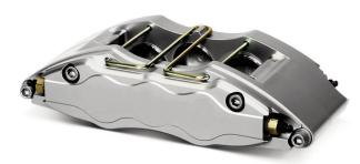
With the fixed calliper there are hydraulic pistons on both sides of the calliper body whereas with the sliding calliper the pistons are only on one side of the calliper body which makes the sliding calliper more compact and lighter.
