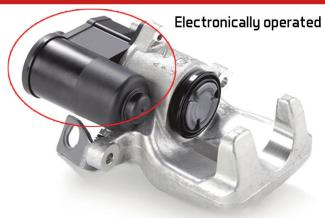
This type of caliper is also used for normal pedal braking and the piston is operated hydraulically. However it is also used to operate the parking brake.
