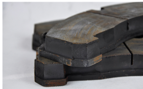
Wear image of Juratek pads and discs after a full weekend of racing
